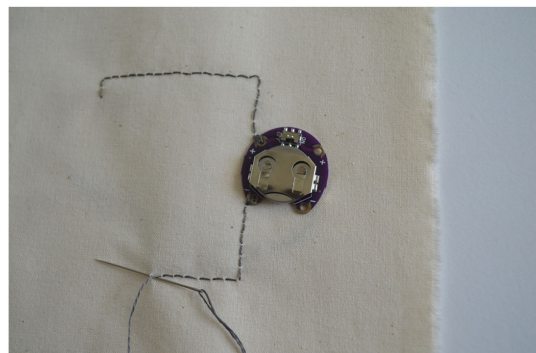
Sew the positive and negative side of the battery holder and leave a long lead of thread for each one
